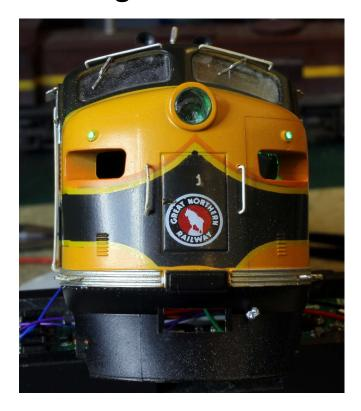
This is a Kato F3 but from memory it is very similar to the Stewart F3. The class lights above are SMD LEDs size 603. The lenses are 1mm Fibre Optic The outer part has had a soldering iron near it to "bell" the lens BEFORE inserting into the 1mm hole. A drop of ACC is applied at the back of the lens. When the glue has set the fibre is cut flush with the inside of the shell.
