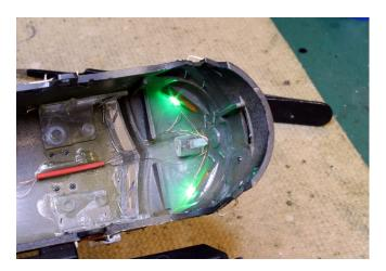
The LEDs are glued to the body to line up with the fibre – again using ACC. The LEDs had the wires soldered on before I got them – the wires are run past the Headlight lens and then down to the heatshrink glued to the roof. This keeps the wires away from the gear tower. The LEDs will be
