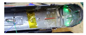
A piece of tape holds the excess wire up out of the way. The wires are soldered to a short piece of PCB Tie glued to the roof. This also has the 3K3 resistor mounted with the LEDs in series. The blue wire goes to the +ve pad on the Tsunami and the and the green goes to an available Fx output. The decoder in this loco is a TSUNAMI 1.
